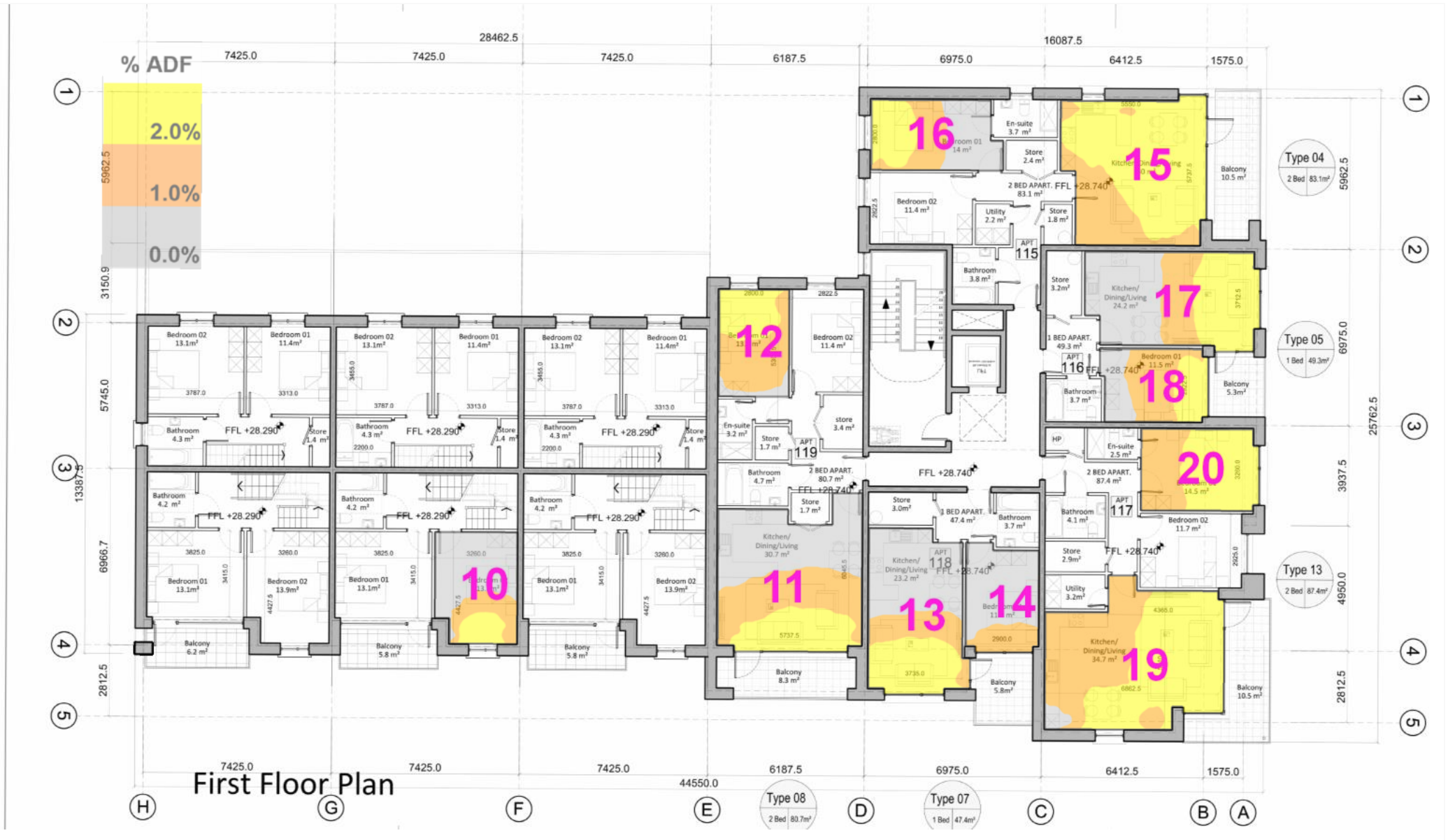
Figure 6 Rooms assessed at Level 01 within Apartment Block 5
