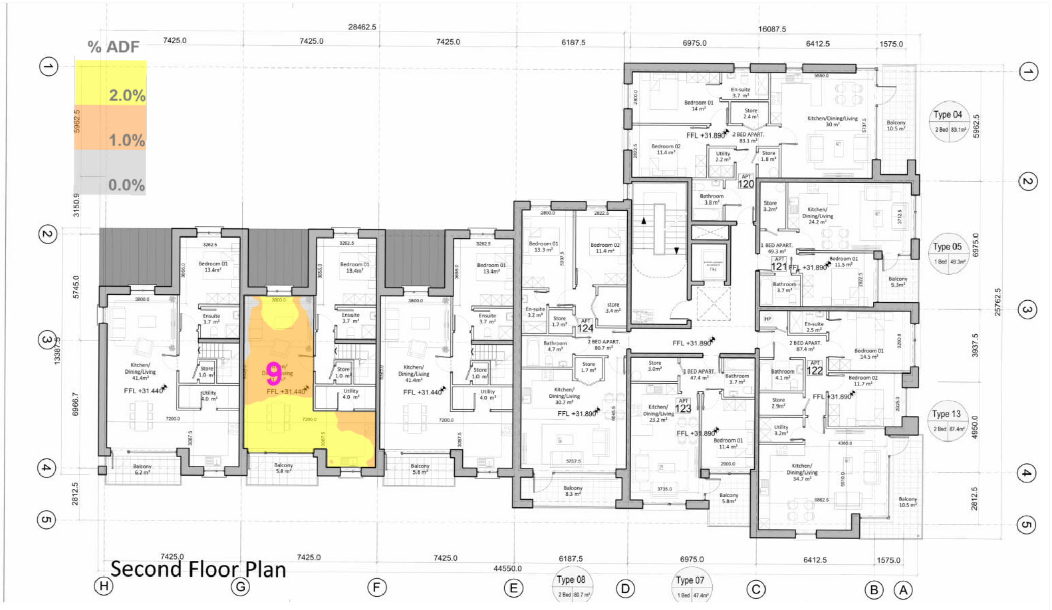
Figure 7 Rooms assessed at Level 02 within Apartment Block 5
