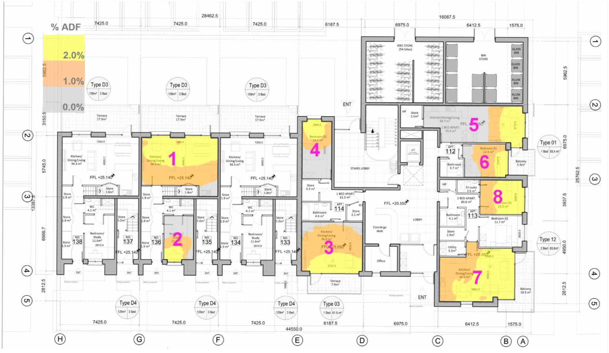
Figure 5 Rooms assessed at Level 00 within Apartment Block 5
